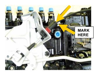
**<u>NOTE:</u>** Disconnecting the cable from the support bracket and the throttle lever is a difficult task; it may be easier to adjust without removing cable.
