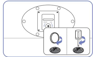
Turn the connecting screw at the bottom of the stand fully so that it is completely fixed.
