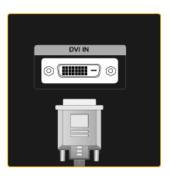
Connect the DVI Cable to the DVI IN port on the back of your monitor.
