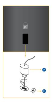
The Kensington Lock is a device used to physically fix the system when using it in a public place. The locking device has to be purchased separately. The appearance and locking method may differ from the illustration depending on the manufacturer. Refer to the manual provided with the Kensington Lock for proper use. The locking device has to be purchased separately.
