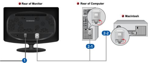
1 Connect the power cord for your monitor to the power port on the back of the monitor.
