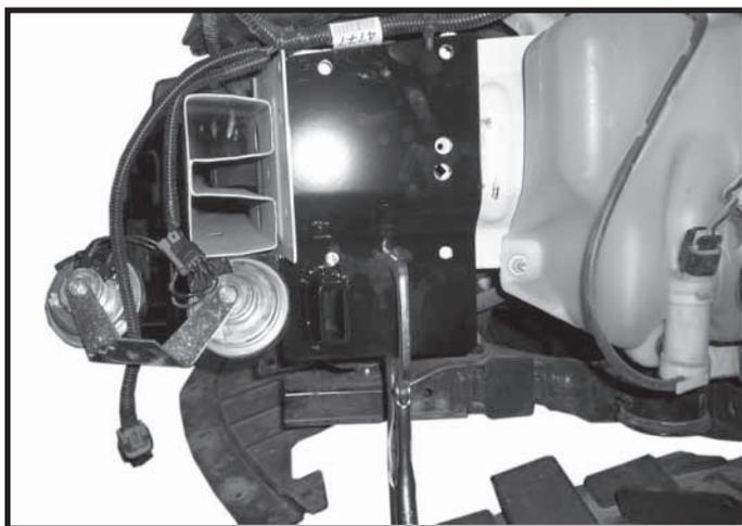
10. With an assistant, slide base plate up onto frame and forward to bumper make sure horn bolt hole and air box holes line up, then clamp.
