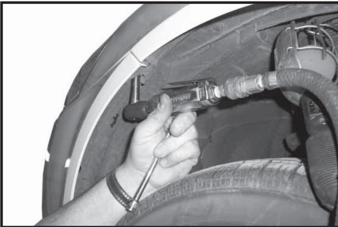
4. Remove one bolt on each side that connects fascia to fender.
