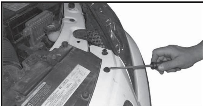
1. Open hood and remove six plastic push fasteners.
