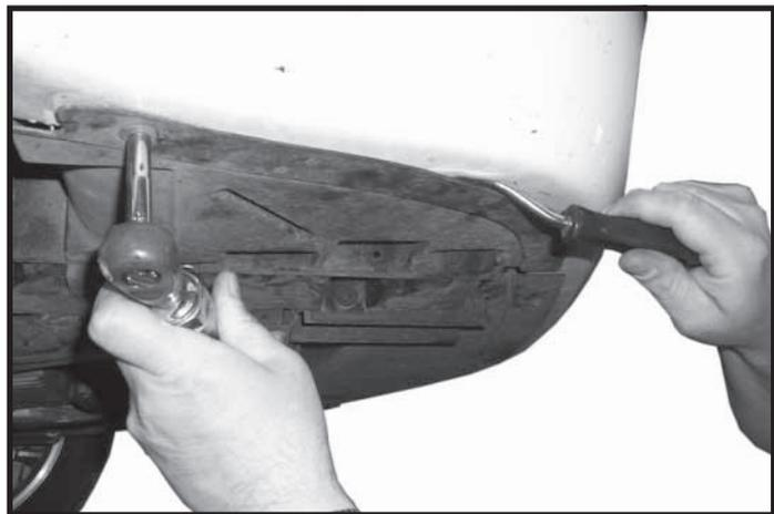
5. Remove four plastic push fasteners and one screw from filler panel on each side.
