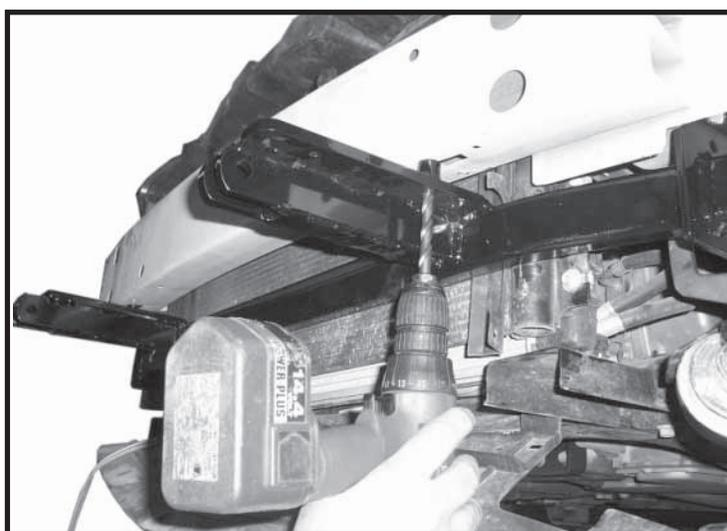
12. Drill two 3/8" holes in bumper using base plate chain anchor as a guide insert bolts and tighten (use shims if needed).
