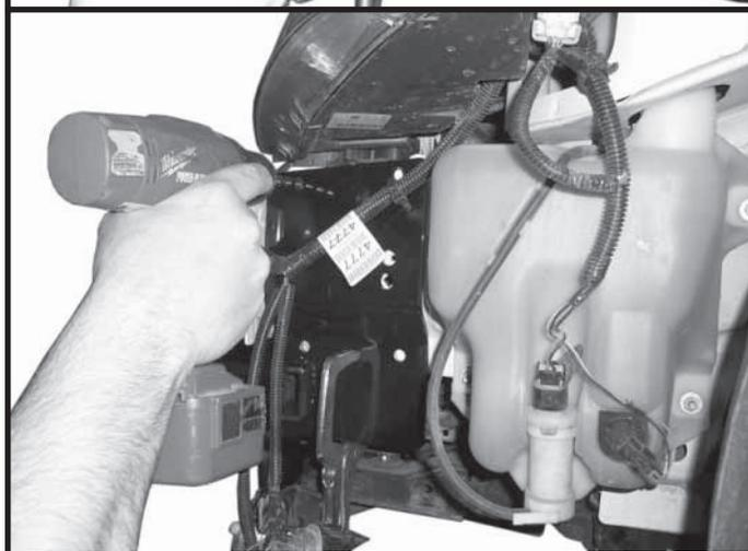
11. Drill bottom two 3/8" holes (on each side) insert bolts and tighten, drill top two 3/8" holes (on each side) place spacer bushings on each as shown on front cover with the longer spacers on the drivers side and the shorter spacers on the passenger side. **NOTE:** Use Blue **LOCTITE**® on threads and tighten bolts according to bolt chart on front page.
