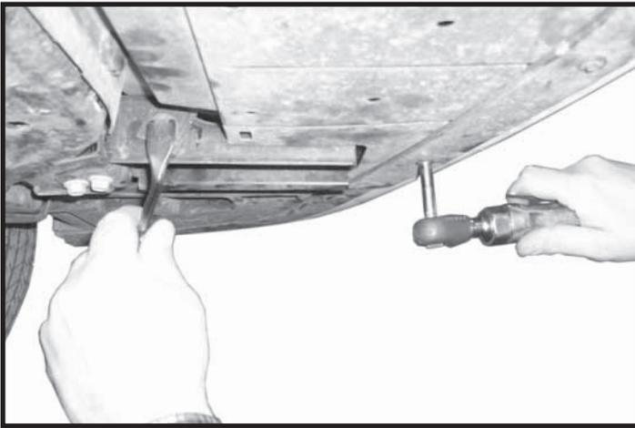
3. Remove plastic filler panel from under fascia by removing five screws and two plastic push fasteners.
