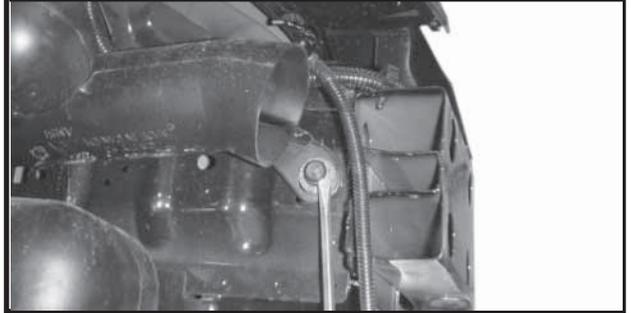
7. Remove air intake on passenger side, by removing one bolt and two plastic push fasteners.
