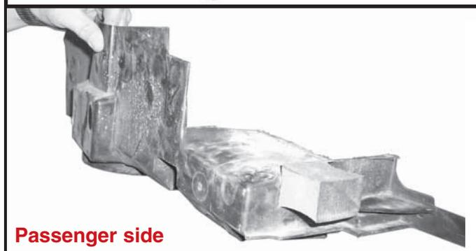
13. Notch plastic filler panel as shown in picture on each side and replace.
