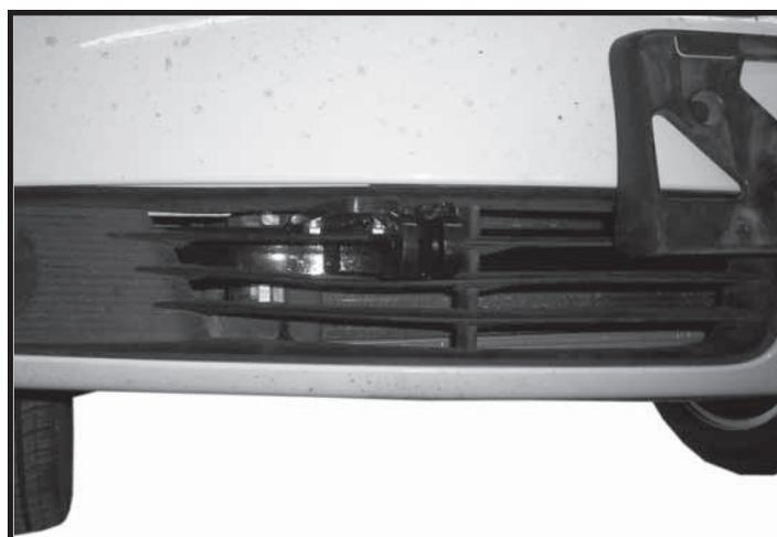
14. Notch plastic on front fascia for pull ears as shown above. Reinstall fascia, plastic filler panels and all hardware. Install horn with longer supplied metric bolt, washer, and lockwasher.
