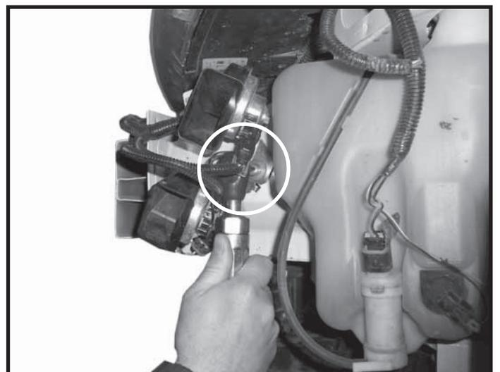
9. Remove one bolt from horn. Bolt will not be reused.
