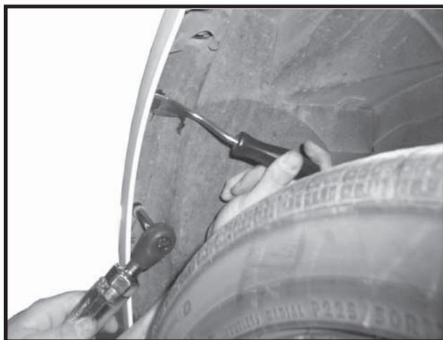
2. Remove three plastic push fasteners and one screw from wheel well on each side.
