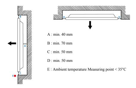
• When embedding the product in a wall, be sure there is some space behind the product for ventilation, as shown above, and maintain the ambient temperature at 35°C or lower.
