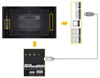
Connect the MAGICINFO terminal on the network box to the HDMI IN2(MAGICINFO) terminal on the product using the MAGICINFO OUT-HDMI cable.
