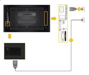
Connect the Power terminal on the product and the Power terminal on the network box to the outlet respectively, using the power cable.
