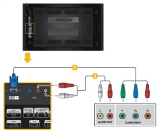
Onnect a RGB to Component cable between the [RGB/COMPONENT IN] port on the LCD Display and the P<sub>R</sub>, Y, P<sub>B</sub> jacks on the Set Top Box.
