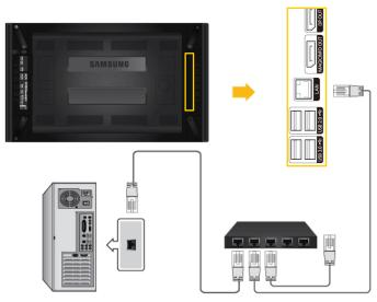
Connect the LAN cable between the [LAN] port on the product and the [LAN] port on your PC.
