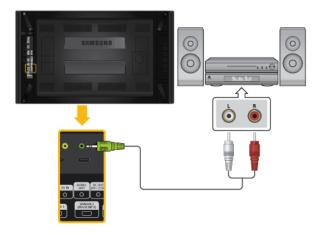
1. Connect a set of audio cables between the AUX L, R jacks on the AUDIO SYS-TEM and [AUDIO OUT] on LCD Display.
