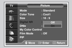
If the signal received by your television is weak, you can activate this feature to help reduce any static and ghosting that may appear on the screen.
