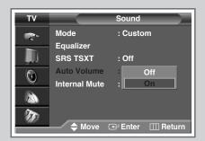
Each broadcasting station has its own signal conditions, and so it is not easy for you to adjust the volume every time the channel is changed. This feature lets you automatically adjust the volume of the desired channel by decreasing the sound output when the modulation signal is high or by increasing the sound output when the modulation signal is decrease.
