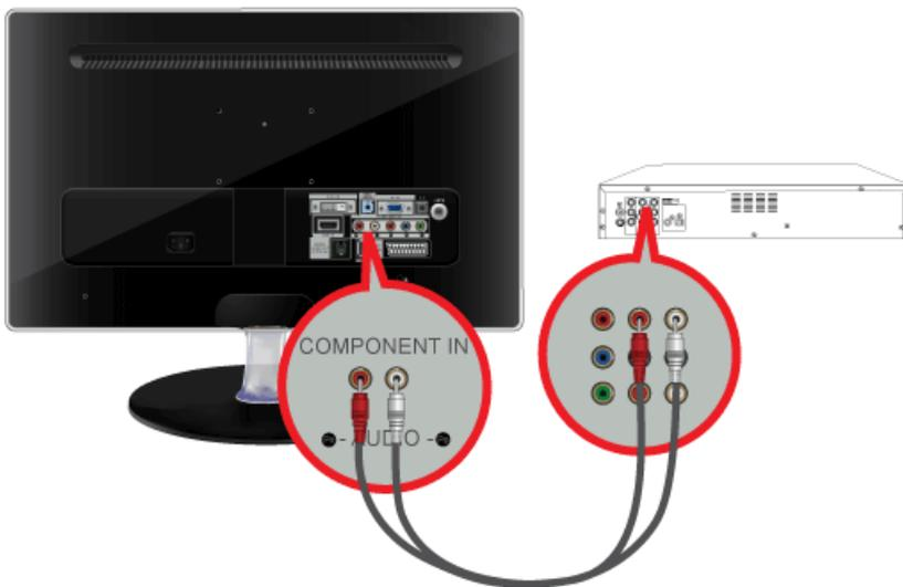
2. Connect the audio port of the AV device (DVD/VCR/Cable/Satellite box) to the [COMPONENT IN [R-AUDIO-L]] port of the monitor.
