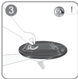
Turn the connecting screw at the bottom of the stand fully so that it is completely fixed.
