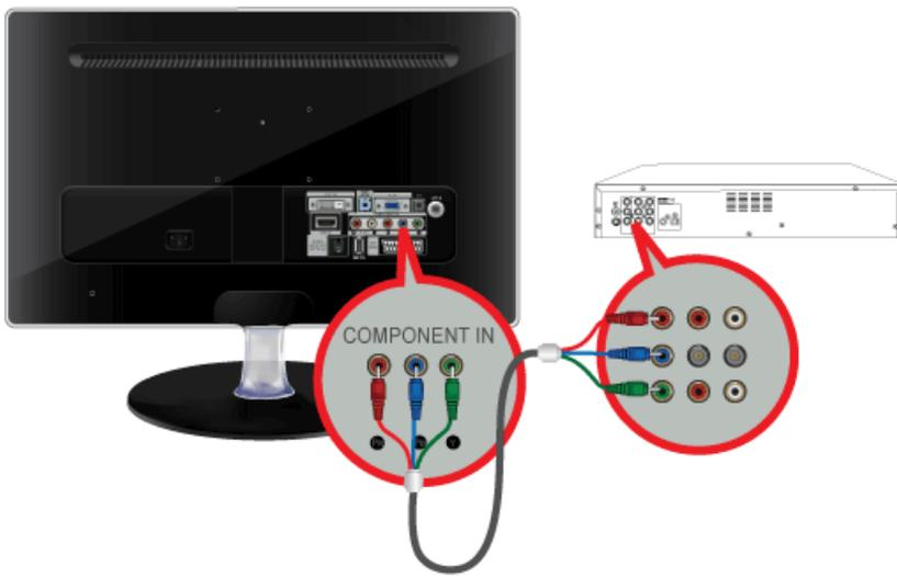
1. Connect the VIDEO OUT port of the AV device (DVD/VCR/Cable/Satellite box) to the [COMPONENT IN [P<sub>R</sub>, P<sub>B</sub>, Y]] input ports using a component video cable [P<sub>R</sub>, P<sub>B</sub>, Y].
