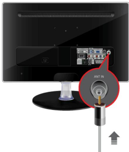
1. Connect the cable/satellite or TV antenna cable to the [ANT IN] port on the rear side of the monitor.
