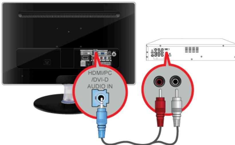
2. Connect the red and white plugs of an RCA to stereo (for PC) cable to the same colored audio output terminals of the digital output device, and connect the opposite plug to the [HDMI/PC/DVI-D AUDIO IN] terminal of the product.
