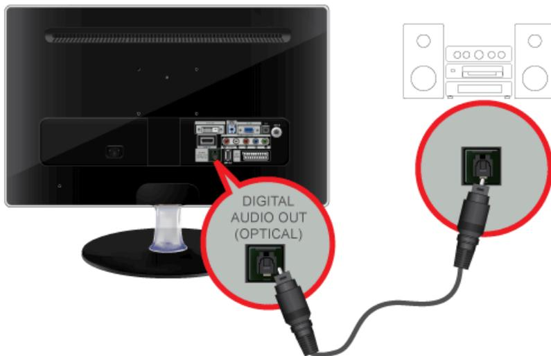
Connect the [DIGITAL AUDIO OUT (OPTICAL)] terminal of your monitor to the optical input of your amplifier using an optical cable.
