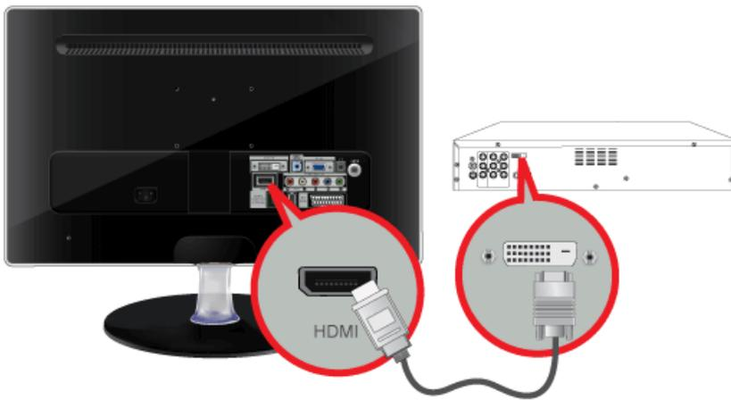
1. Connect the DVI output terminal of an external device to the [HDMI IN] terminal of the monitor using a DVI to HDMI cable.
