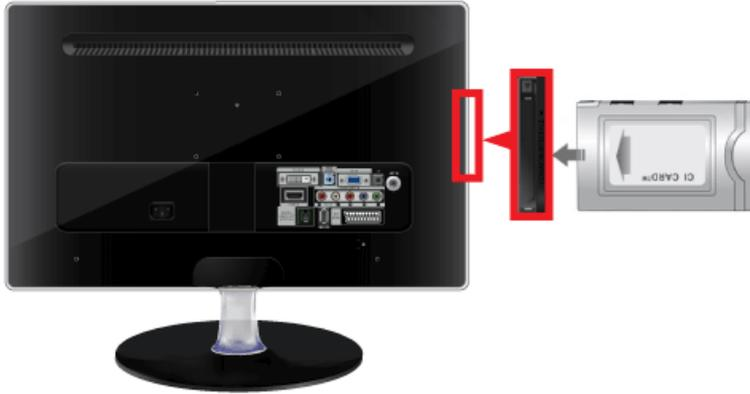
1. Insert the CI CARD into the CAM in the direction of the arrow until it fits.
