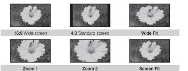
Screen Fit Displays the full image without any cut-off when HDMI (720p / 1080i / 1080p) or Component (1080i / 1080p) signals are inputted.
