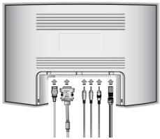
Connect the cables as shown in the picture.
