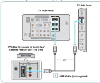
Connect an HDMI Cable between the HDMI IN (1, 2, 3 or 4) jack on the TV and the HDMI jack on the DVDJBu-Ray player or Cable Box/Satellite receiver (Set-Top Box).
