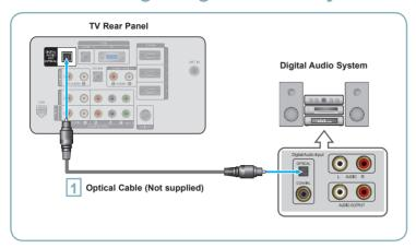
Connect an Optical Cable between the "DIGITAL AUDIO OUT (OPTICAL)" jacks on the TV and the Digital Audio Input jacks on the Digital Audio System.
