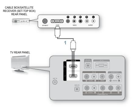
1. Connect an HDMI Cable (Not supplied) between the HDMI IN (1 or 2) jack on the TV and the HDMI jack on the Cable Box/Satellite receiver (Set-Top Box).
