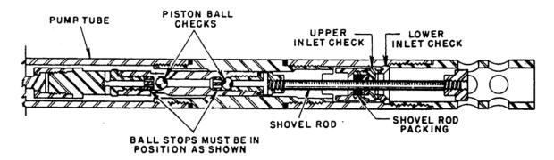
Loss of pressure, volume or continuous operation of pump when not in normal use indicates:
