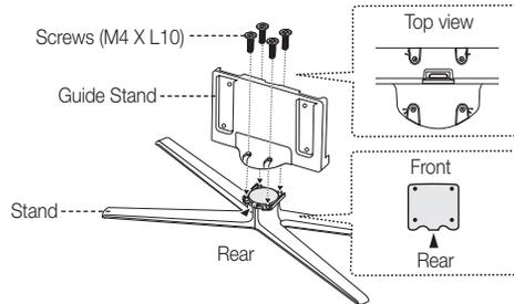
1. Connect the Guide Stand to the Stand using four screws (M4 X L10) as shown.
