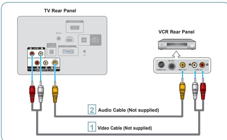
**1** Connect a Video Cable between the AV IN [VIDEO] jack on the TV and the VIDEO OUT jack on the VCR.
