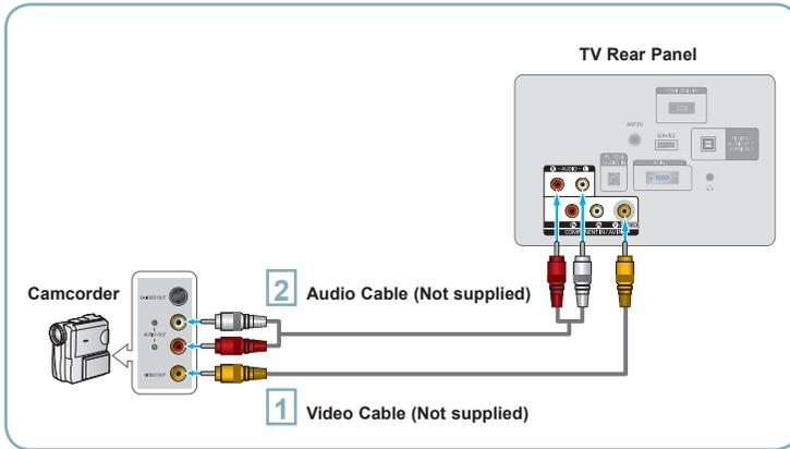
**1** Connect a Video Cable between the COMPONENT IN / AV IN [VIDEO] jack on the TV and the VIDEO OUT jack on the camcorder.
