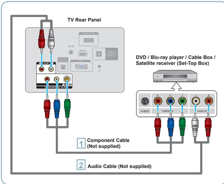
**1** Connect a Component Cable between the COMPONENT IN [ Y, P<sub>B</sub>, P<sub>R</sub> ] jacks on the TV and the COMPONENT [ Y, P<sub>B</sub>, P<sub>R</sub> ] jacks on the DVD / Blu-ray player / Cable Box / Satellite receiver (Set-Top Box).
