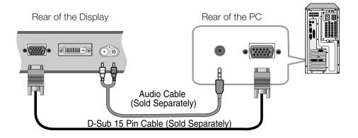
Figure 3-3. Analog RGB Connections
