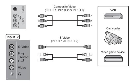
Figure 3-5. Composite and S-Video Connections
