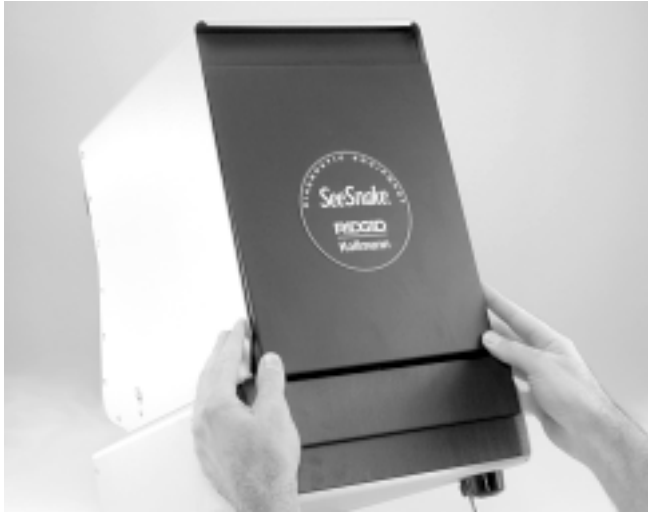
Figure 5 – Completely Closing the Top Door
