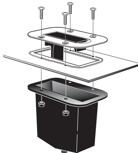
3. If installing Pole Holder only: Place Pole Holder into cutout and fasten with four #8 flat head self-tapping stainless steel screws.
