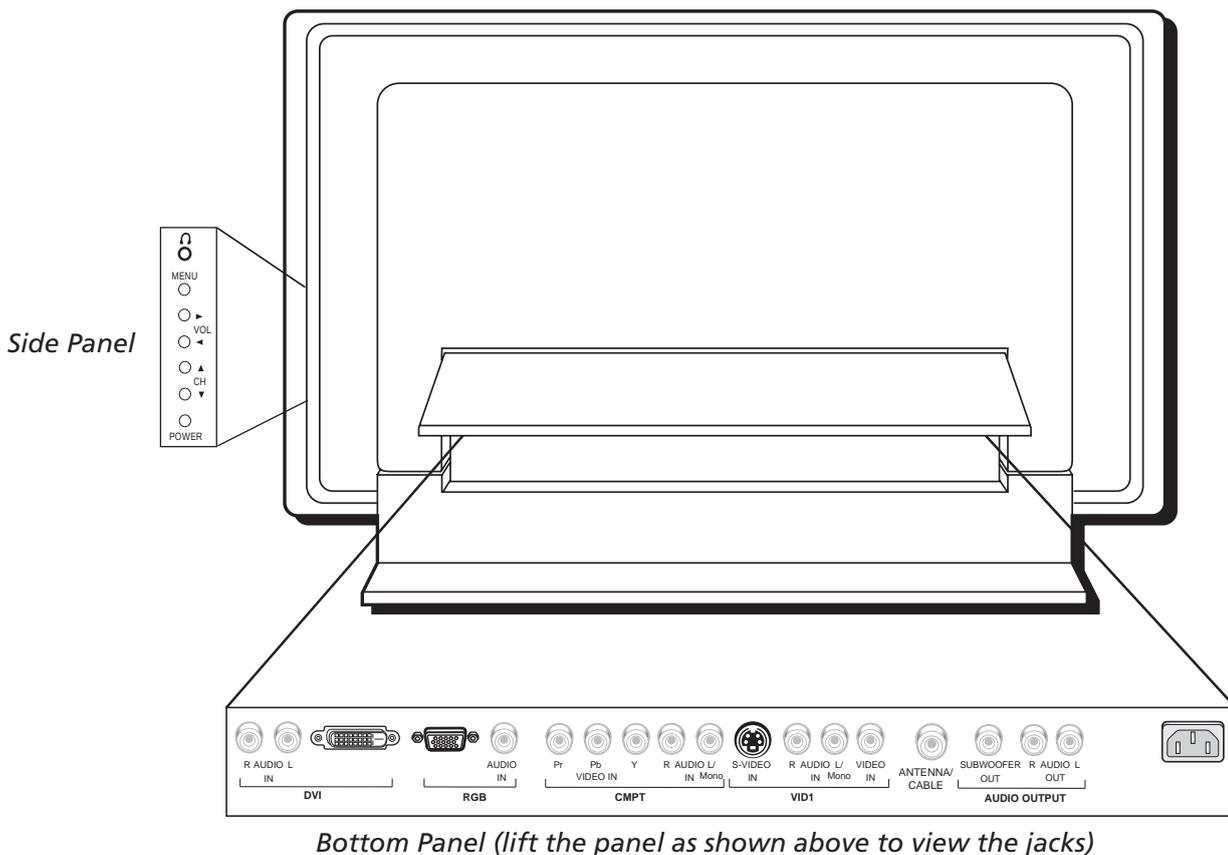
*Bottom Panel (lift the panel as shown above to view the jacks)*
