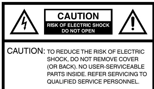
The lightning flash with arrowhead symbol, within an equilateral triangle is intended to alert the user to the presence of uninsulated dangerous voltage within the product's enclosure that may be of sufficient magnitude to constitute a risk of electric shock.
