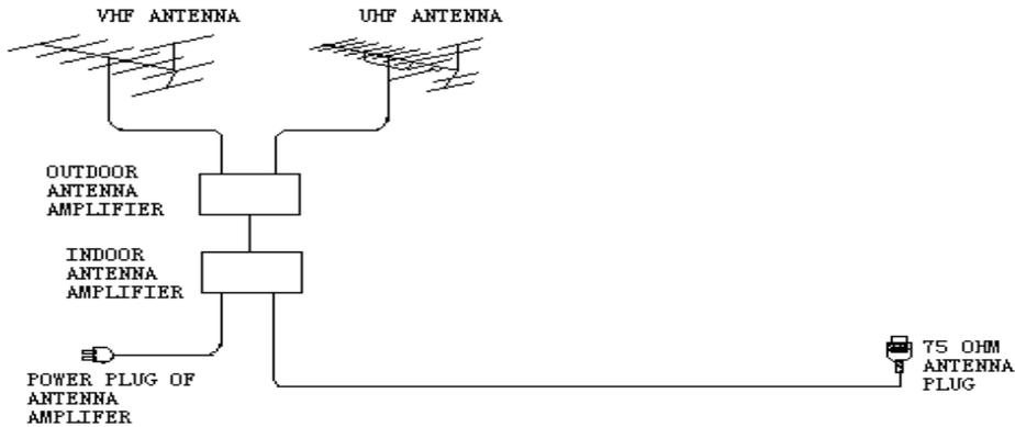
To ensure good picture and sound, TV antenna system needs to be installed. The antenna system as shown can be sourced from TV equipment shops, which will provide service for correct installation and connection. After installation, insert the 75-ohm antenna plug into the antenna jack as shown. In case of signal of closed circuit TV,
