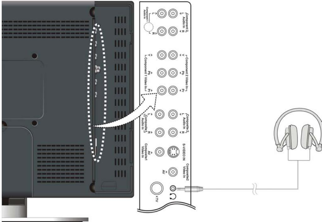
When earphones are connected, the television will automatically mute internal speaker output.
