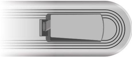
Insert two batteries (1.5V, size AAA), ensuring the polarity matches the marks inside the compartment.
