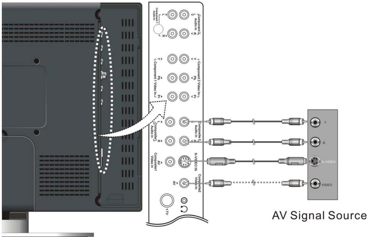
After connection, turn on the power of the unit and the external AV signal source and use the Input button to select AV2 (Composite) mode.
