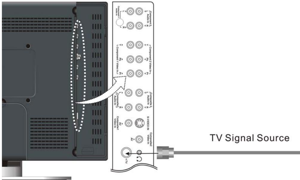
After connection, turn on the power of the unit and use the Input button to select TV mode.
