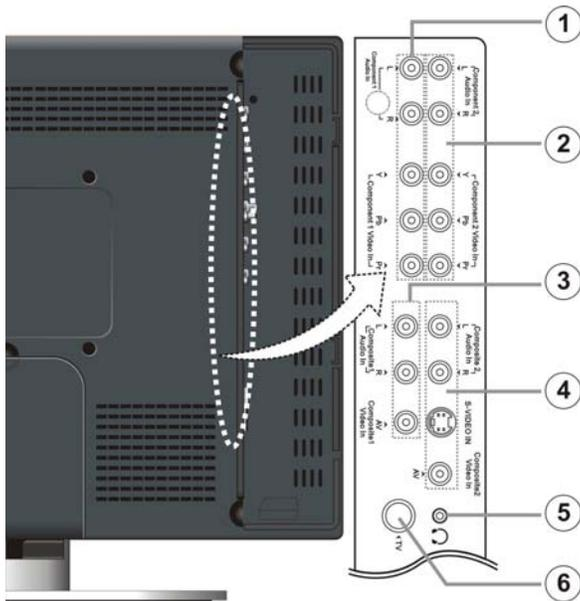
**1. Y/Pr(Cr)/Pb(Cb) (Component) and L/R audio Input Jacks**
