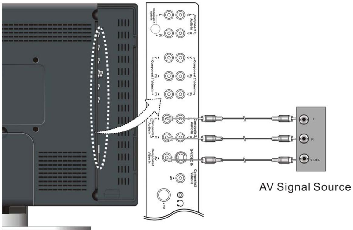
After connection, turn on the power of the unit and the external AV signal source and then use the Input button to select AV1 (Composite) mode.
