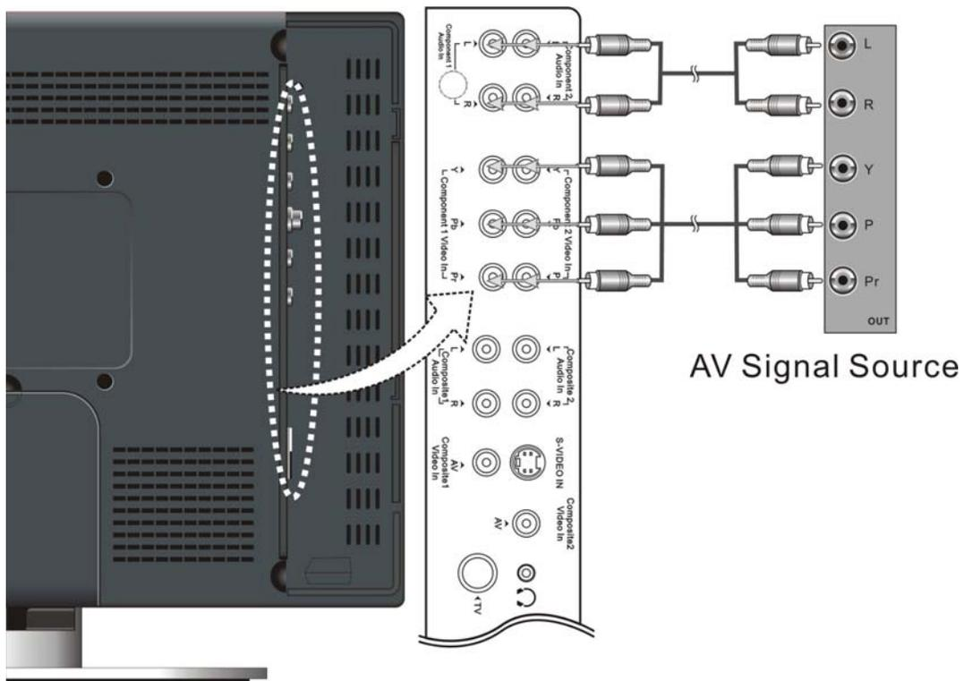
After connection, turn on the power of the unit and the external AV signal source and press the Input button to select AV3 (Component) or AV4 (Component) mode.
