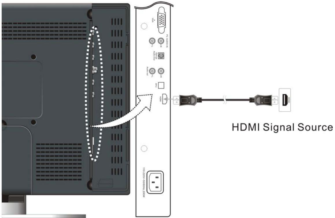
After connection, turn on the power to the television and the external HDMI device and use the Input button to select HDMI mode.
