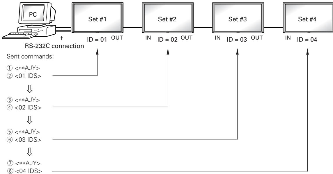
By sending RS-232C commands in this order, it is possible to assign an ID for each unit.
