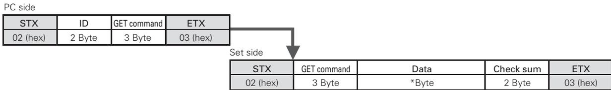
Example) Check Sum value that is added when the GET command [GAA] returns the following 6-Byte data
