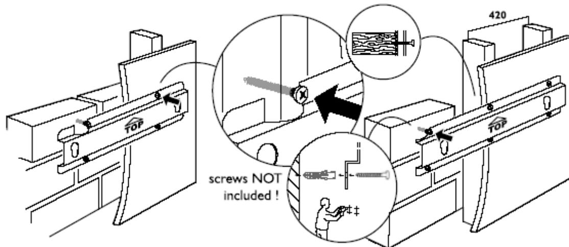
2. Secure the Mirror TV onto the Wall mount bracket, as shown:
