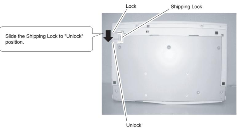
1. Raise the scanner carefully upward so that bottom side of the scanner faces towards you.
