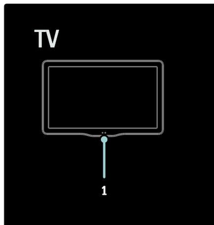
1. **Ambient sensor / remote control sensor**
