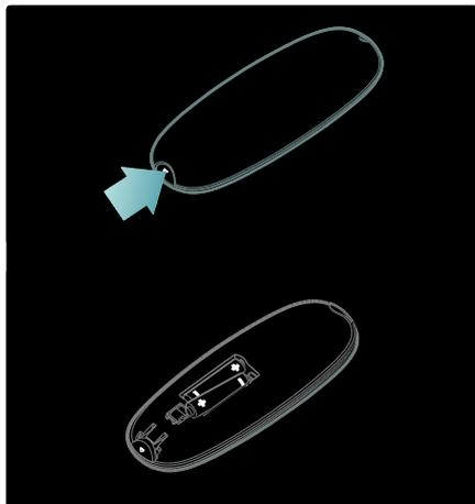
For remote control with CR2032 (3V) batteries:
