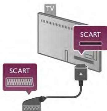
Use the supplied SCART adapter cable to connect your device.
