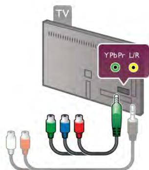
Use the supplied YPbPr adapter cable to connect your device. Match the YPbPr (green, blue, red) connector colours with the cable plugs when you connect.
