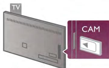
Use the Common Interface slot on the TV to insert the CAM card\*. Gently insert the CAM as far as it will go and leave it in the slot permanently. It may take a few minutes before the CAM is activated. Removing the CAM will deactivate the broadcast service on TV.
