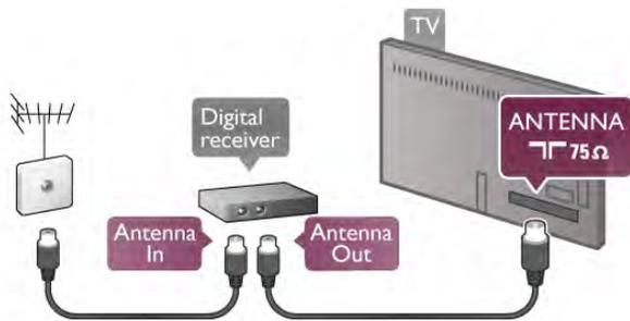
Next to the antenna connections, add an HDMI cable to connect the Set-top box to the TV. Alternatively, you can use a SCART cable if the Set-top box has no HDMI connection.
