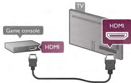
If the game console is connected with HDMI and has EasyLink HDMI CEC, you can operate the game console with the TV remote control.
