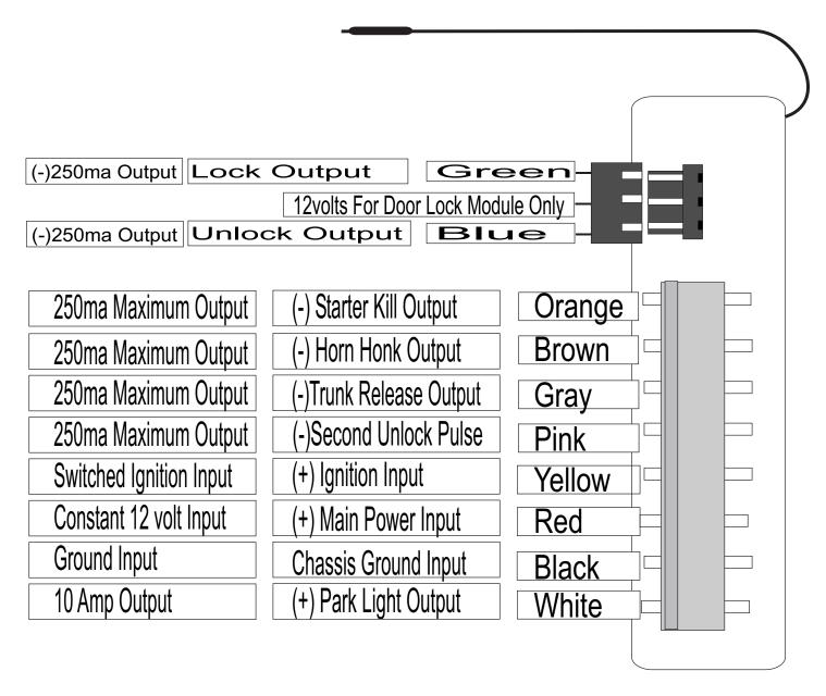
\*The 12volt output on the keyless entry connector is not to be used for anything other than suppling power for voltage inverter's, and door lock modules such as the DL-3 and DL-7.
