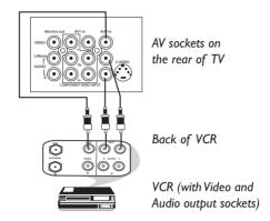
You can view the playback of VCR tapes (Video Disc players, camcorders, etc.) by using the AUDIO and VIDEO INPUT sockets on the rear of the TV.
