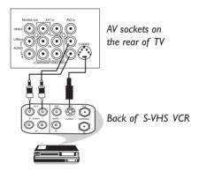
The S-Video connection on the rear of the TV is used for the playback of S-VHS VCR tapes, Video Discs, Video Games or Compact Disc-Interactive (cd-i) discs. Better picture detail and clarity is possible with the S-Video playback as compared to the picture from a normal antenna (RF) connection.
