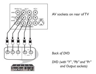
You can view the playback of DVD discs by using the COMPONENT VIDEO INPUT (CVI) sockets on the rear of the TV.
