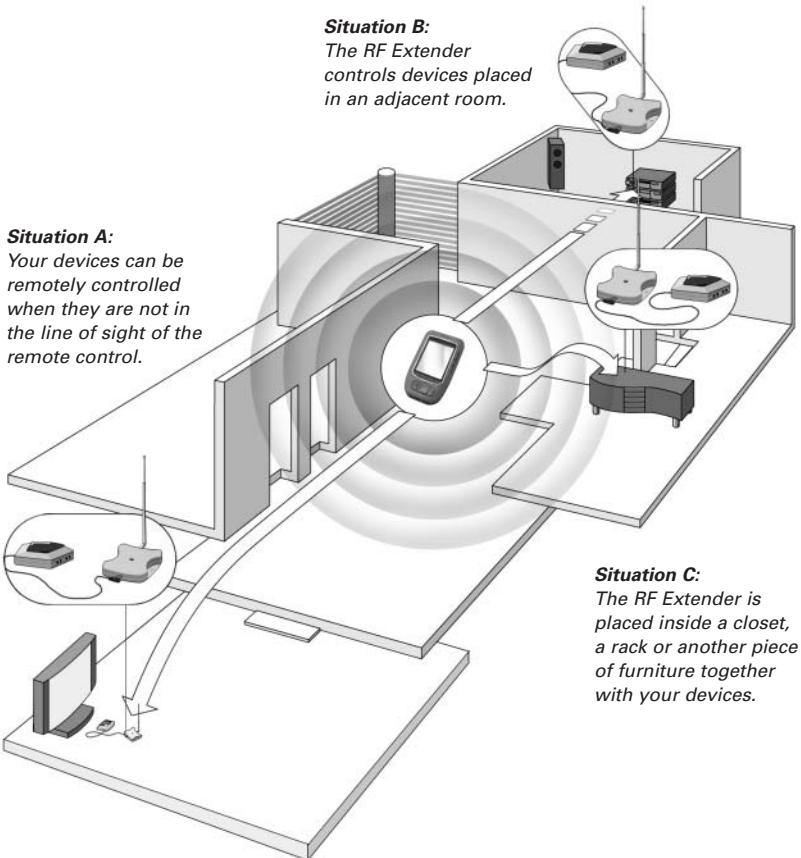
The arrangements in the situation shown above can also be combined. You can control all RF Extenders individually with one or more Pronto Remote Controls.
