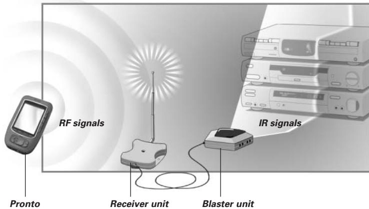
When the Blaster unit cannot reach all devices or transmits with too much power, you can use the included **Dual IR emitters**. You can set up the Dual IR emitters in two ways:
