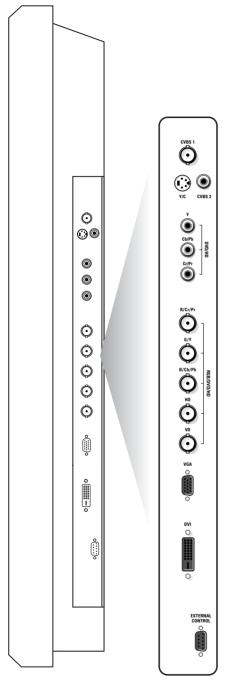
You may connect 2 possible VGA sources (VGA or RGB Digital (DVI)) and 3 possible video sources (AV1, AV2 and AV3) to the right side of the monitor.
