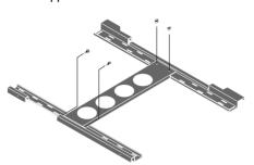
Pasten the unit with commercial anchors or the four screws. Be sure that the anchors or screws are fastened at a position where there is a post.
