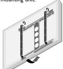
Fit the upper hooks of the display fittings into the grooves of the (upper) wall fittings and adjust for level positioning.
