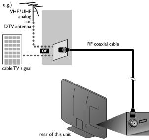
Once connections are completed, turn on the unit and begin initial setup. Channel scanning is necessary for the unit to memorize all available channels in your area. [Initial Setup] - p.15
