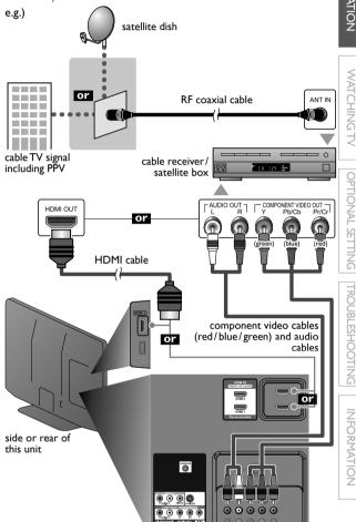
You can also connect this unit to the cable receiver or satellite box other than the HDMI or the component video output jacks because they might have different output jacks.
