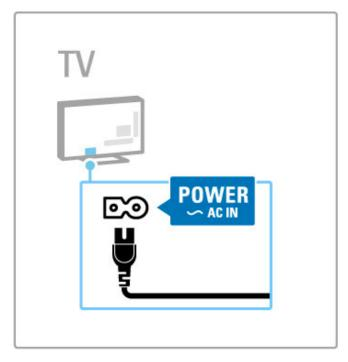
Although this TV has a very low standby power consumption, switch off the TV with the power switch to save energy if you do not use the TV for a long period of time. Read more about the power switch in  $Help > Getting \ started > Keys \ on the TV > Power \ switch.$
