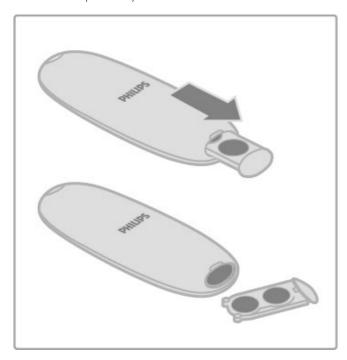
Remove the batteries if you are not using the remote control for
