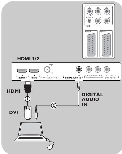
**PC equipped with a DVI connector:**
