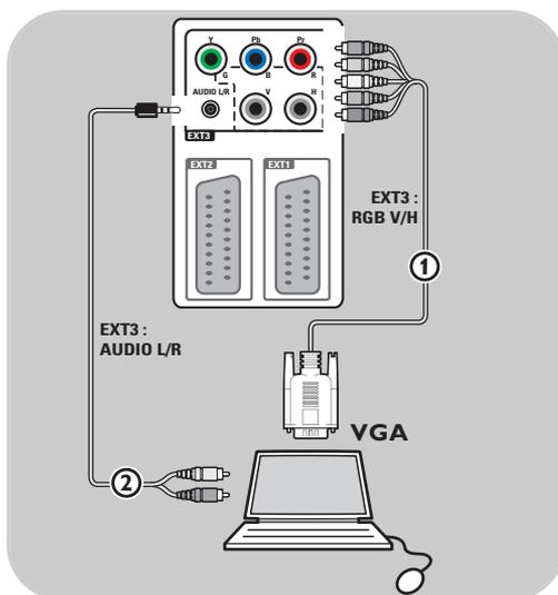
**PC equipped with a VGA connector:**
