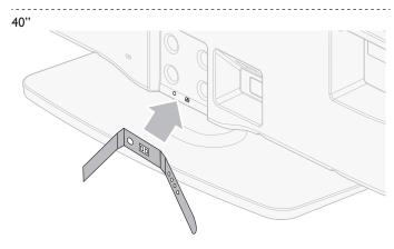
2 Pass cables through the cable management tie to avoid tangles. 55"/46"
