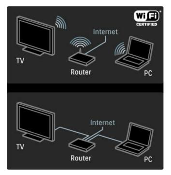
If you use a wired connection to the router you need a network (Ethernet) cable.
