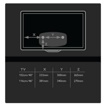
Fix the 2 mounting discs. Use screws with a diameter of max 6mm.
