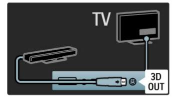
${\bf 3}$  Install the 3D transmitter on the top or at the bottom of the TV. Make sure to point the transmitter directly to where you sit to watch TV.
