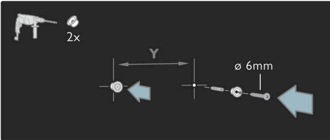
Slide the bottom plate of the stand onto the mounting discs.
