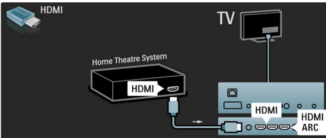
If you use the HDMI-ARC connections on both TV and device, no other cable is needed. If not, read on.
