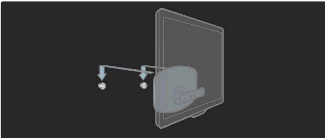
To level the TV, pull the bottom of the TV towards you slightly and let it slide on the discs.
