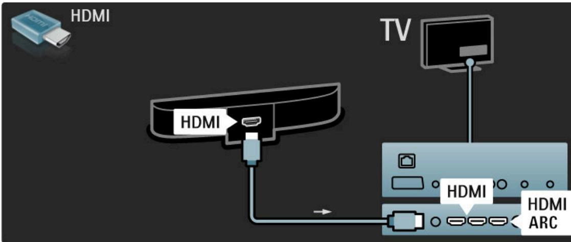
If you do not use the HDMI-ARC connection, add a digital audio cable (cinch coaxial).
