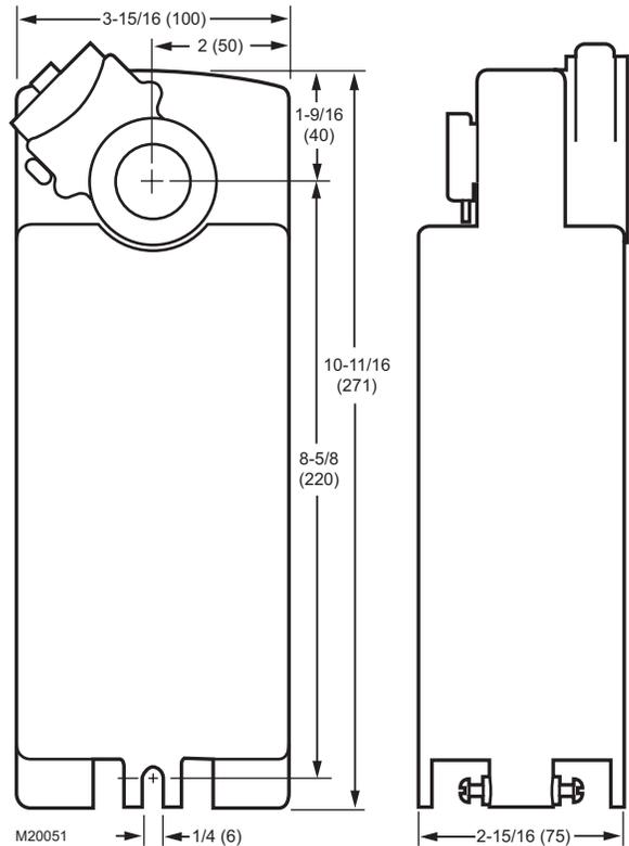
**Fig. 1. Dimensional drawing of actuator in inches (mm).**
