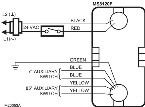
Fig. 6. Typical 24 Vac wiring (MS Series).
