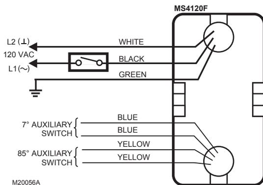
Fig. 7. Typical 120 Vac wiring (MS Series).
