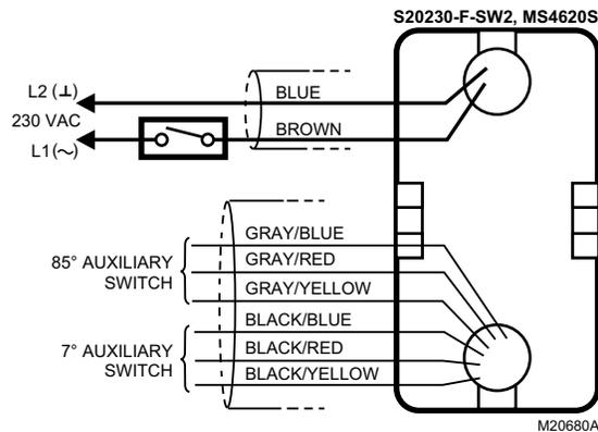
Fig. 10. Typical 230 Vac wiring (S20 Series).
