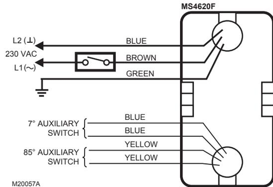
Fig. 8. Typical 230 Vac wiring (MS Series).
