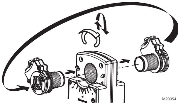
Fig. 4. Mounting shaft coupling to actuator opposite side.
