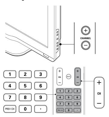
Press CHANNEL +/- on the side of the TV. For digital channels, press a number (1 to 135) followed by a dot "•" and then the corresponding sub channel number (1 to 135). e.g. 108.30.
