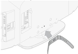
Pass cables through the cable management tie to avoid tangles.
