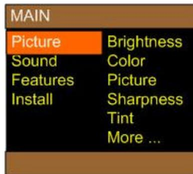
The primary use of this menu is to program the digital channels using the Auto Program function of the digital module in the television. To program the digital channels, cursor down to Install, and Cursor Right. This will display the Install Menu. From The Install menu, select Auto Program and Cursor Right to start the Auto Programming.
