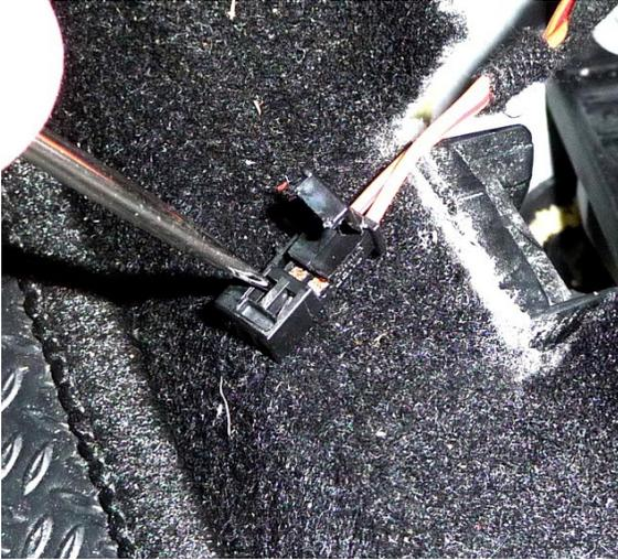
Remove pins from connector housing
