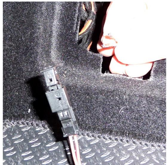
Pins ready for new connector housing
