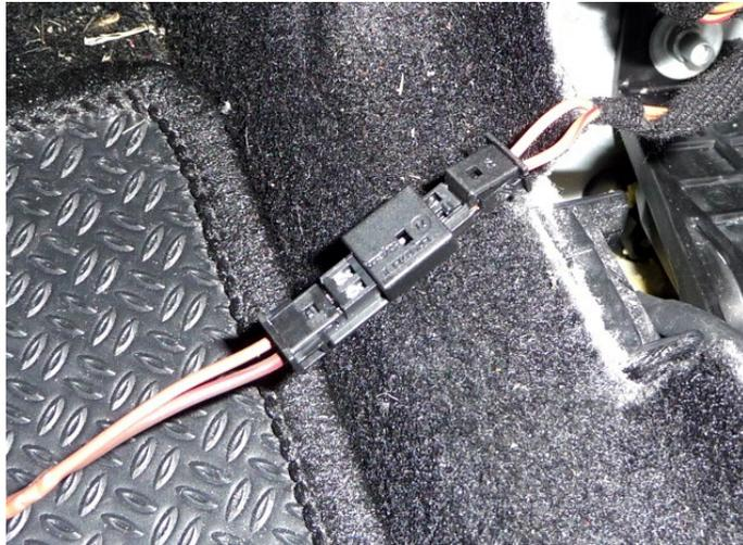
Pins installed in connector housing
