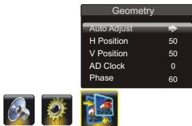
**Auto Adjust:** press the right direction or OK button to adjust the picture's position, phase and clock automatically. The menu will auto exit after the adjustment is finished..
