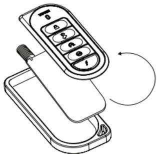
2. Turn both the unit front and circuit board over, remove battery from clip and replace.
