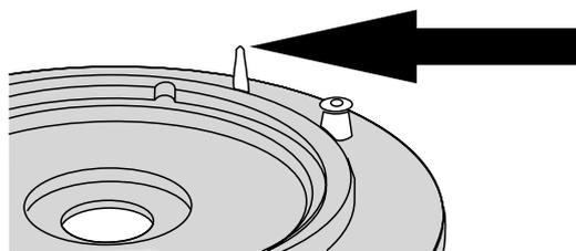
*If you have lifted up the hotplate then carefully replace it taking care not to damage or displace the ignition electrodes or flame safety probes (arrowed) and replace the rear fixing screws.*
