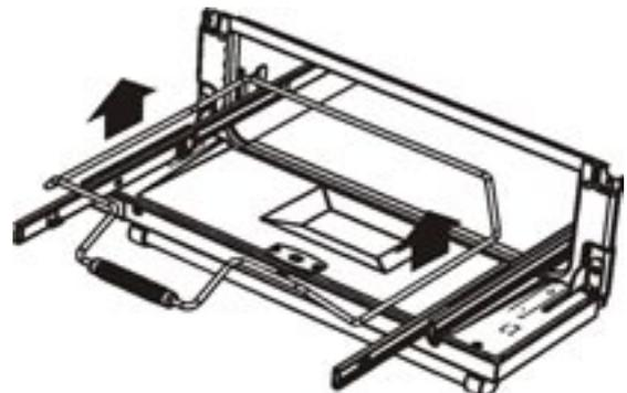
For safety, push the side rails into the grill chamber.
