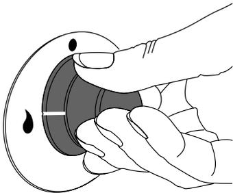
Keep holding the knob pressed in to let the gas through to the burner for few seconds. The igniter should spark and light the gas.
