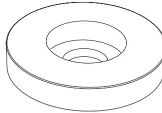
*If you are converting to LP Gas the burner ring in the centre burner must be changed for the large ring in the conversion kit.*
