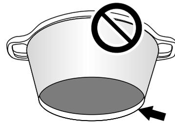
Pans and kettles with concave bases or down turned base rims should not be used.
