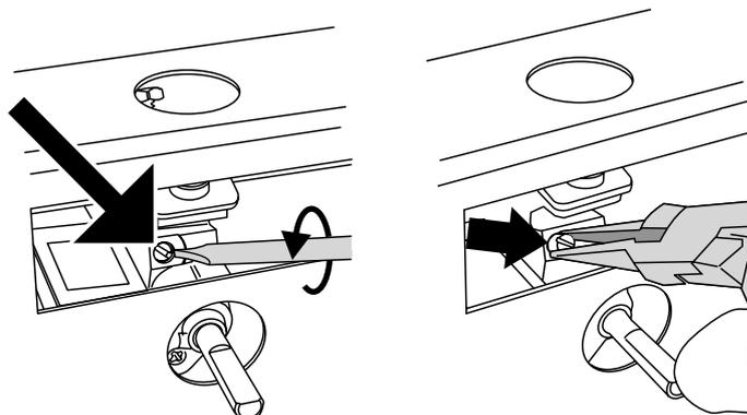
*The tap bypass screw is now accessible. Unscrew the tap bypass screw.*
