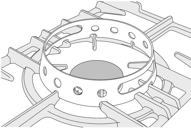
It should be located so that the cut-outs in the ring sit directly on the projecting burner supports.
