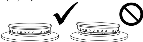
Check burner ports are not blocked. If blockage occurs, remove stubborn particles using a piece of fuse wire.
