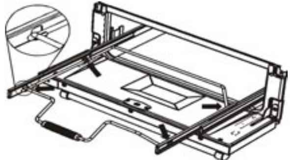
For each side, support the side rail with one hand and with the other hand lift the frame up and out of the side clips.
