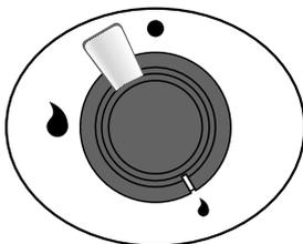
On this cooker the low position is beyond high, **not** between high and off. The small flame marks the 'low position'. Turn the knob towards it after the contents of a pan have boiled.
