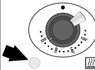
The oven indicator light will glow until the oven has reached the temperature you selected. It will then cycle on and off during cooking.
