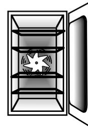
The fan in the right hand oven circulates hot air continuously, which means faster more even cooking.
