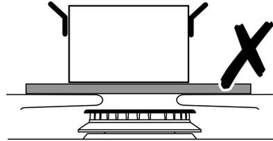
Simmering aids, such as asbestos or mesh mats, are NOT recommended. They will reduce burner performance and could damage the pan supports.
