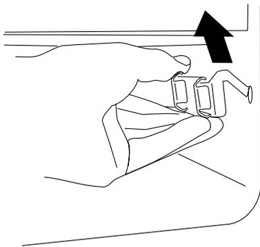
When you have finished, hook the side rails back on to the sides of the chamber. To refit the frame pull the side rails forward and for each side in turn, support the side rail and press the frame down into the side rails.
