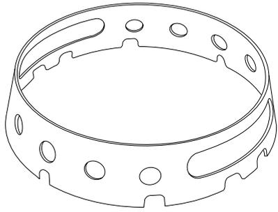
The Wok ring is designed fit the centre burner. It will not fit any of the other burner pan supports
