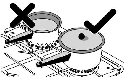
Make sure flames are under the pans. Using a lid will help the contents boil more quickly.
