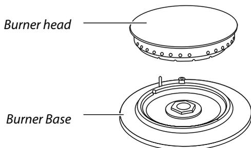
When fitting burner head, ensure this locates properly within the base.
