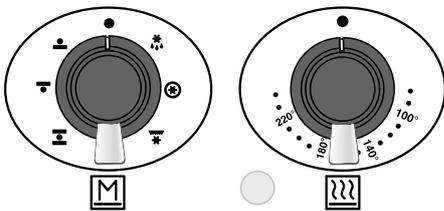
The Multi-function oven has two controls, a function selector and a temperature setting knob.
