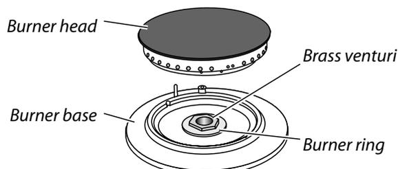
*Undo the large brass nuts and remove the brass venturis and brass rings.*
