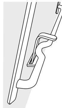
To refit the side support, first locate the tag at the bottom of the support in the slot in the locating bracket in the oven side.
