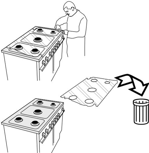
There may be blemishes visible on the stainless steel when the protective coating is removed. This can be caused by moisture and condensation during storage. We recommend cleaning the stainless steel with Kuhn Rikon's 'Swiss Cleaner'.
