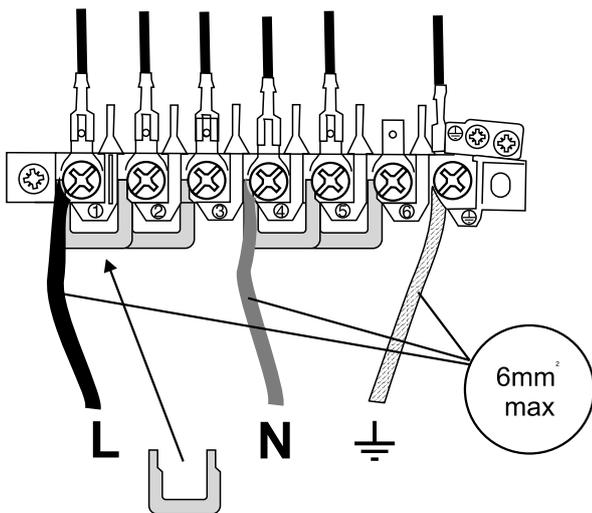
**Check that the links are correctly fitted and that the terminal screws are tight.**
