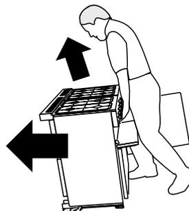
Do not use the door handles or control knobs to manoeuvre the cooker.
