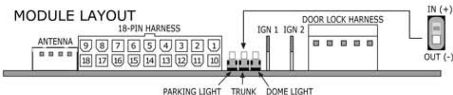
**CAUTION:** Please check the position of the switch before the wire connection is made. You may cause damage to the control module if the incorrect switch polarity is chosen.
