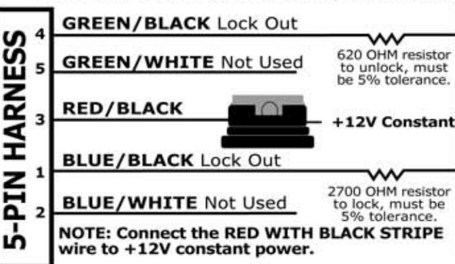
This is an example only. Resistor values and 12V or ground may vary depending on make and model of the vehicle.
