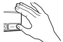
4. Release buttons when the motor unit lights blink. It has learned the code. If light bulbs are not installed, two clicks will be heard.
