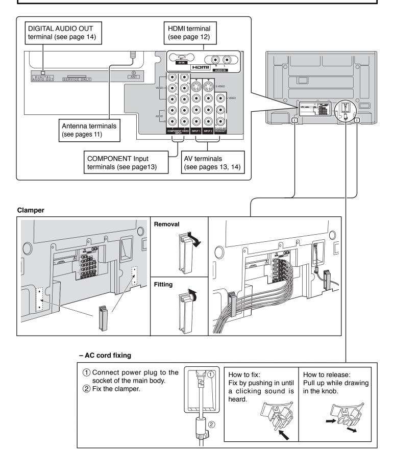
Note: To avoid noise do not put the Antenna cable and AC cord together.
