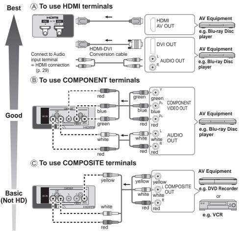
The Green terminal is shared for both the COMPONENT and COMPOSITE (VIDEO IN) connection. When using COMPOSITE (VIDEO IN) connection, the Yellow connector (Video) should be inserted into Green connection. (Watching content from external devices (p. 19))
