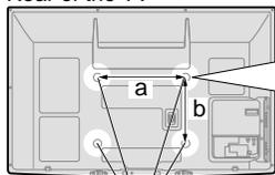
Holes for wall-hanging bracket installation
