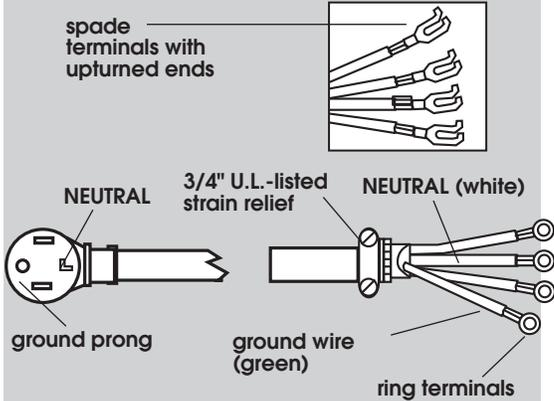
Four-wire power supply cord must have four, No.-10 copper wires and match a four-wire receptacle of NEMA Type 14-30R. The fourth wire (ground conductor) must be identified with a green cover and the neutral conductor by a white cover.
