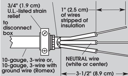
Strip 3-1/2" (8.9 cm) of outer covering from end of cable. Strip insulation back 1" (2.5 cm). If using 3-wire cable with ground wire, cut bare wire even with outer covering.
