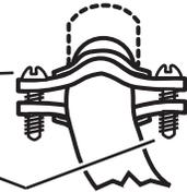
**8.** To exhaust dryer, see Exhaust requirements, Pages 3-4. Connect exhaust vent to dryer exhaust outlet and exhaust hood using 4" (10.2 cm) clamps. Use caulking to seal exterior wall opening around exhaust hood.
