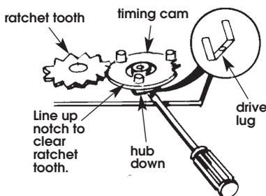
3. Insert a narrow, flat-blade screwdriver under the timing cam near the clock shaft. Gently lift cam straight up and off shaft making sure that the "V"-shaped notch clears the ratchet tooth.
