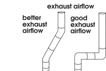
**Four-inch (10.2 cm) metal exhaust vent** is required. Plan installation to use the fewest number of elbows and turns.
