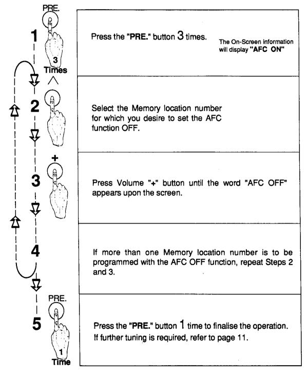
To Reset the AFC function repeat this process and set the AFC ON.
